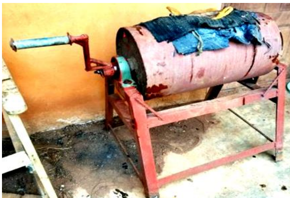
Plates 14: The Completed and Assembled ball mil
