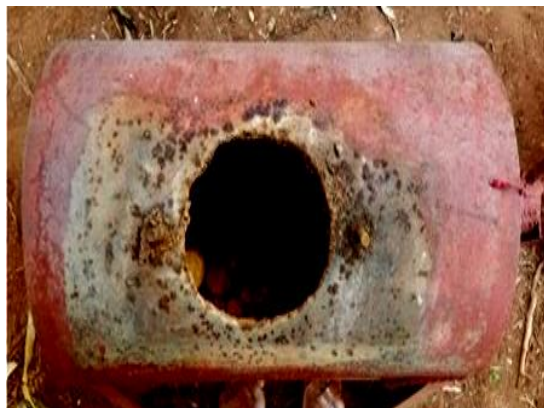
Plate 8: The cylinder tank with 16mm opening at the center
