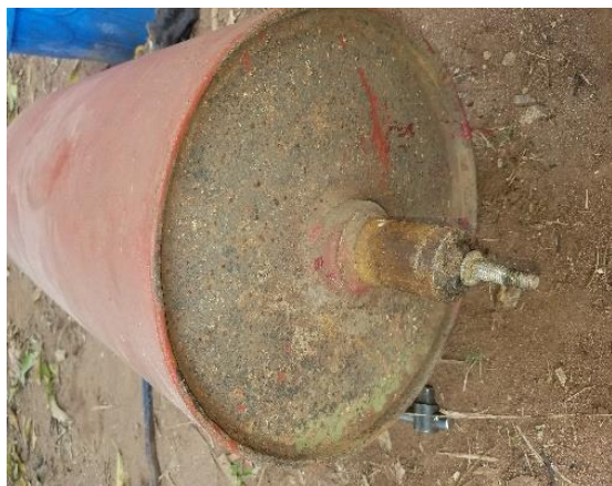
Plate 7: The cylindrical tank with the flat pans welded To cover the sides and the shaft passing through the center
